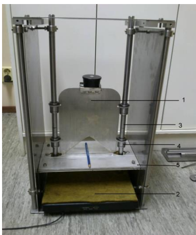
Figure 1. The test device to determine the shear energy of meat by using GIM method (1 – blade, 2 – force transducer, 3 – blade leading rods, 4 – slidebearing, 5 – cutting table).
