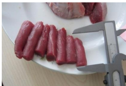
Figure 3. Samples of meat taken by hollow drill.
